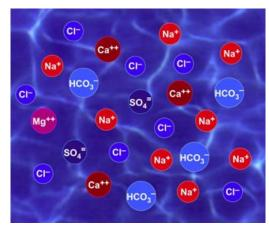
magnesium ions will not bind with the carbonate anions in the water. So there is no formation of scale. This technology will not remove the calcium and magnesium ions from the water, but instead changes their chemistry so that they can remain in the water but not negatively affect hard surfaces that they come in contact with, such as your plumbing, hot water heater, fixtures, dish washer, washing machine, shower, tub, or any other water using appliances.
